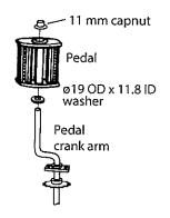
Place pedal crank over edge of workbench or table, as shown. Using the capnut driver supplied, hammer capnut onto end of pedal crank. Repeat Subassemblies A and B.
